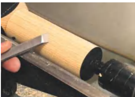
▲ Pic.13 The spindle roughing gouge will not leave a great finish, especially on pine. The skew is now presented with the centre of the tool cutting and the bevel rubbing
